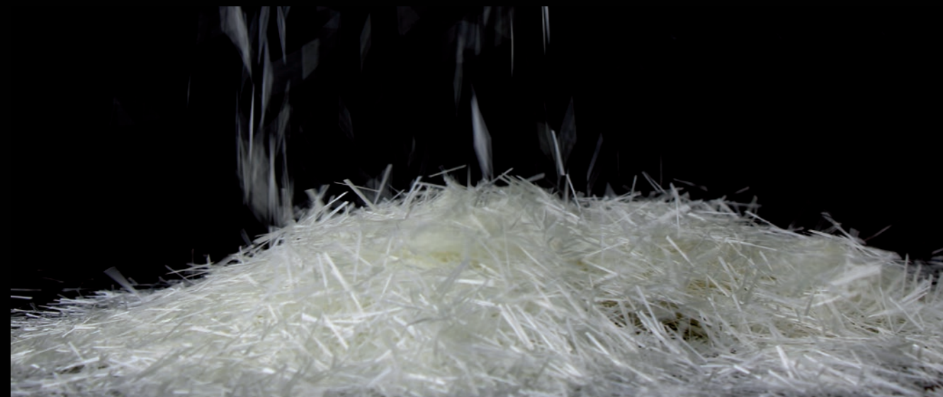
Mascot's alkali resistant glass fibre: cut to size and weighed in each batch to ensure quality
