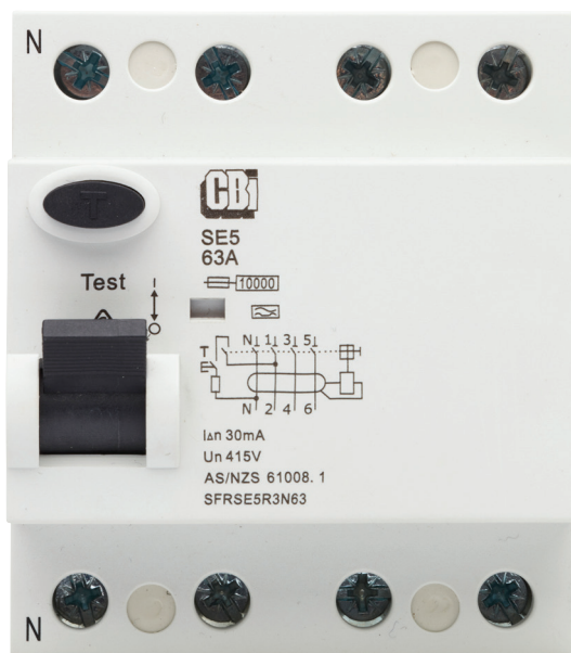
SFRSE5 | Residual Current Circuit Breaker | 3 + N | 6 kA
