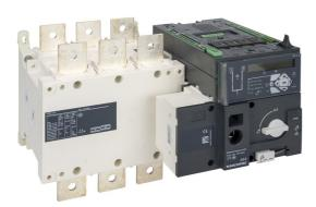
ATyS P 125A 4 pole basic transfer switch - integrated transfer logic, LCD display with energy/power metering, comms
