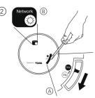
switch Master and all Slave alarms ON. Note: Take care when inserting screwdrive
