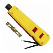
This impact type punch down tool is used for telecommunication and network installations. The one motion action presses the cable into an insulationdisplacement connector and neatly snips off the cable end. Adjustable high and low actuation setting accommodates termination requirements or user preference.
