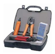
The kit includes everything you needed to install and terminate network cables. The tool kit comes in a plastic tool box with carry handle. The tool kit includes crimp tool, cable stripper and 110 punch down tool.
