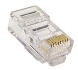
Similar to the standard 8 position modular plug but has raised key on one side of the plug to prevent insertion into a non-keyed 8 position socket. Plugs with 50µ", 30µ" or 15µ" gold plated contacts are available. Packed in bags of 20, 50, 100 or 1000. Plugs for stranded or solid conductors with round or flat cord entry are available.
