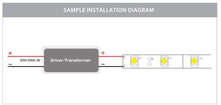
Must be used with a suitable 12v DC LED Driver
