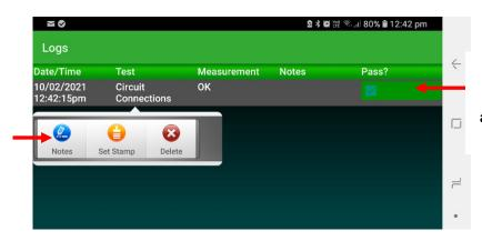
Tap the "Pass?" column tick box to mark the log entry as PASSED (green) or FAILED (red).
