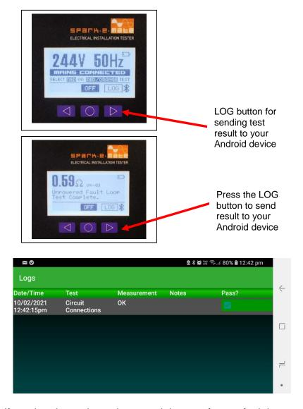
Please note that if you log the mains voltage and then perform a fault loop test, Spark-e-Log will automatically calculate and log the <u>Prospective Short Circuit Current (PSC)</u>.
