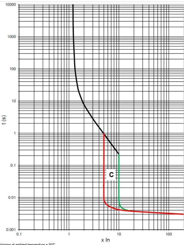
Thermal tripping at ambient temperature = 30°C In = RCBO rated current
