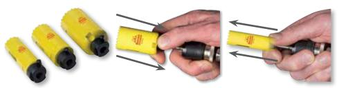
Push the button on the arbor and pull the hole saw down the pilot drill. To use a new hole saw, push the button on the arbor and slide the hole saw forward to remove it.
