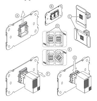
Note: The Dual Port Charging Mechanism body is wider on one side than the Single Port mechanism. This restricts the multi-gang capacity for Dual Port mechanisms to 2.
