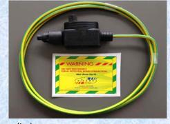
**APPLICATION:** The reinforcing mesh can be cut in the wet area location and the WETCON™ secured over one of the cut ends. This is achieved by tightening the shear bolt with the recommended spanner until it snaps off ensuring the correct tension of the connection.
