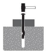
Tap in anchor until seated and flush with surface of fixture.
