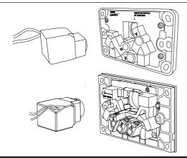
1. 30USBCM with standard clip into twin socket 2025 / C2025.
