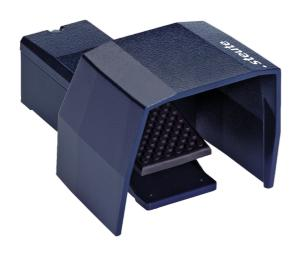
GF Series Foot Switch, Aluminium Die-cast Enclosure with screw connection terminals, with protective shield, slow action with double break, 2 NC/2NO contacts, 6A/400V AC switching current, EN ISO 13849-1; EN 60947-5-1
