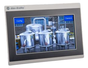
PanelView 800 7 inch HMI, Touch Screen Serial and Ethernet ports
