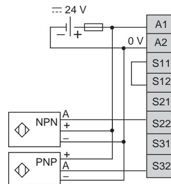
**NOTE:** The sensors must be supplied by the same PELV/SELV power supply as the safety module.
