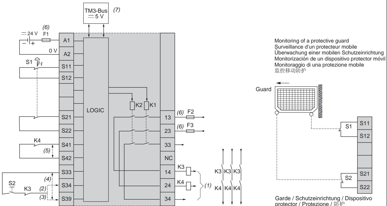
S1 = EMERGENCY STOP / Bouton poussoir d'ARRÊT D'URGENCE / Not-Halt / PARADA DE EMERGENCIA / ARRESTO DI EMERGENZA / 紧急停止.
