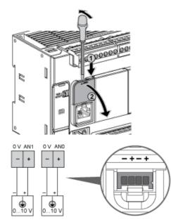
The (-) poles are connected internally.
