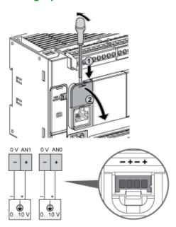
The (-) poles are connected internally.
