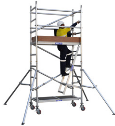
CONFIGURATION 2 PLATFORM HEIGHT 2.3m Base Pack + Extension Pack + Ladder + Horizontal Bracing + Toe Boards + Outrigger Pack
