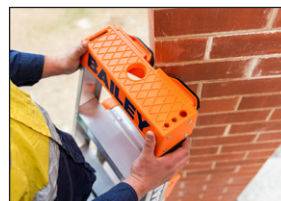
Outside corner leaning
