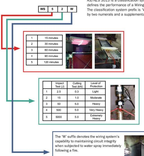
Cables are subjected to fire at 1050°C for 120 minutes, then water sprayed for a further 3 minutes.
