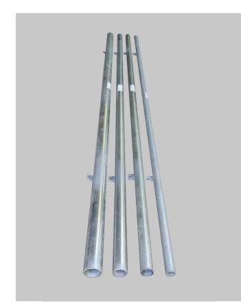
Used to protect various size conduit and cable coming from underground up the side of a stobie pole. 2500 long. Manufactured using AS/NZ Standard Grade Galvanized Medium Steel plain end pipe.
