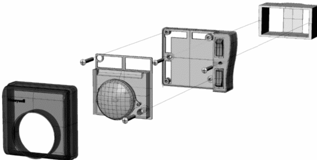
Fig 3: Horizontal Installation diagram
