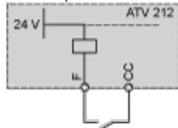
“PLC” position with PLC transistor outputs
