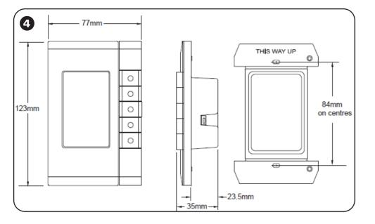
The Saturn eDLT wall plate cannot be used until it is programmed by the installer or integrator using C-Bus Toolkit software. C-BusTookit can be downloaded free from the Internet at the following URL:
