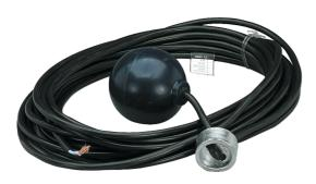
Float Switch, 67mm diameter, minimum switching depth 100mm, minimum voltage 6V DC, maximum voltage 240V AC, maximum operating current 2A, maximum 100 Va, 10m cable, 1 NO contact
