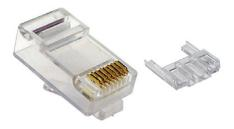
These special plugs are designed for Category-6 cables. Special contact design allows the same plug to be used for either solid or stranded conductor cables. The 2-piece design includes a cable-guide to ensure conductors are split into 2-rows to maintain data integrity. 50µ" gold plated contacts.
