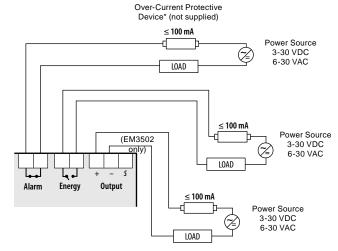
The solid state pulse outputs are rated for 30 VAC/DC nom.
