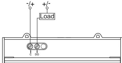
**en** The digital output is polarity-independent.
