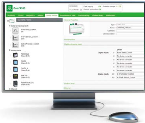
Device settings page (partial), as displayed after auto-discovery, enabling user to assign circuit identifications and select data for logging and publication.
