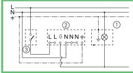
This wiring example shows the switch installed with a single switch. The switch needs to be closed for normal sensor operation.
