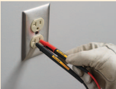
Increase tip exposure for CAT II probing
