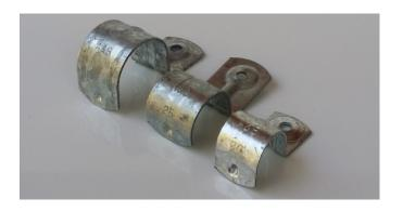
Made to clamp various sizes of conduit to any surface using Tek screws or nails. Manufactured using AS/NZ Standard Grade Z275 Galvanized Steel.
