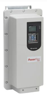
PowerFlex 753 AC Drive, 400 V AC, 3 PH, 72 A, 37 kW ND, 30 kW HD, Wall Mount - IP54, NEMA/UL Type 12, No Brake Resistor, Blank (No HIM)
