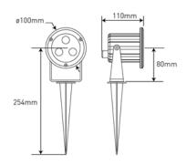
This IP65 rated fitting utilises the latest energy efficient high power LED technology combined with very high quality materials to produce a multi-application product suitable for wall or spike mounting options indoor or outdoor. Used in domestic, commercial, retail, bars, restaurants, leisure and hotels; its applications include illumination for:
