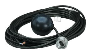
Float Switch, 67mm diameter, minimum switching depth 100mm, minimum voltage 6V DC, maximum voltage 240V AC, maximum operating current 2A, maximum 100 Va, 15m cable, 1 NC contact
