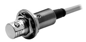
Inductive Proximity Sensor, 3-Wire DC Standard Barrel, 30mm Diameter, Unshielded, Tubular:Stainless Steel, Metal Face, 15mm Sensing Distance, N.O., Source (PNP) Output, ToughLink Cable
