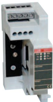
The EP010 Fieldbus interface allows SACE Tmax XT circuit-breakers to be integrated into communication systems to control and supervise using the most diffused communication protocols, such as Profibus, DeviceNet and CANopen (besides ModBus RTU, supported by Ekip Com).
