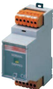
PR212/CI is an interface device that allow Ekip M-LRIU to comand the contactor. The stand-by position normally corresponds to the opening position of the main contacts. PR212/CI can be used in conjunction with XT2-XT4 circuit-breakers equipped with the electronic trip unit for Ekip M-LRIU motor protection.
