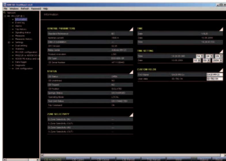
Ekip Connect automatically scans the RS-485 bus, detects all the devices connected and checks their configuration, checking all the possible address, parity and baud rate combinations. A simple click over SCAN will highlight:
