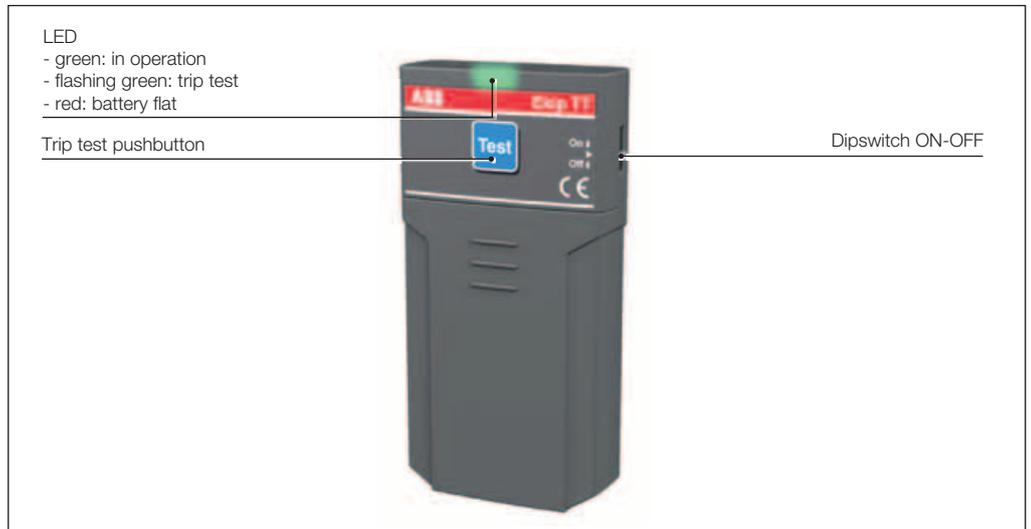
The Ekip TT accessory is supplied with a special connector which makes connection between the electronic trip unit and the Ekip TT unit easier. The kit also include an adaptor which allows use of the Ekip TT unit with the current Tmax breakers.
