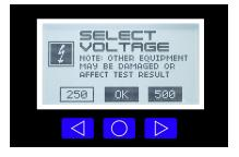
250V d.c. or 500V d.c. nominal is then applied between the selected conductors, in this case Active and Earth. The leakage resistance between Active and Earth is then automatically calculated. This is displayed on the LCD display in KiloOhms ( $K\Omega$ ) or MegOhms ( $M\Omega$ ). A reading of about 1  $M\Omega$  or more is a good result.
