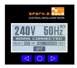
Although the *Spark-e-mate* fascia suggests a test order as per AS/NZS 3000 Clause 8.3.4 Sequence of Tests, the tests can be performed in <u>any order</u> without the risk of damaging the unit. Apart from over-voltage (>300 V a.c.), there are no wiring transpositions or key presses that can damage Spark-e-mate.
