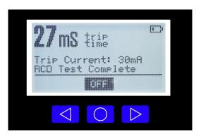
If the RCD fails to trip or the circuit is not protected by an RCD, the LCD will read **RCD TRIP FAILURE**, RCD did not trip.
