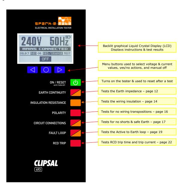
Testing is easily performed from the power point (socket outlet) under test simply by plugging the unit in, pressing the ON/RESET button and selecting a test. The LCD ( $\underline{L}$ iquid  $\underline{C}$ rystal  $\underline{D}$ isplay) then provides a test result.
