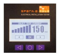
After pressing the OK button shown above, you will receive the final warning that the RCD could trip at the selected firing angle and trip current:
