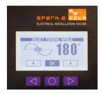
This is the point in the a.c. waveform that the trip current is applied:
