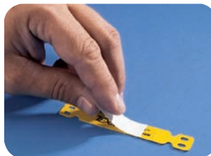
3. Seal the carrier by placing a finger on the foil and pushing forward, thus rolling over the foil and rolling off the silicon liner.
