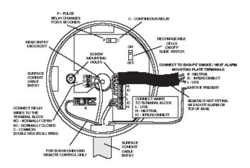
Be very careful about correctly wiring the alarms as mixing Live and Neutral will blow/damage interconnected alarms
