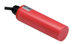
VR Series Capacitive Proximity Sensor, thermoplastic polyester 1 1/2" PT housing, 20 to 30 V DC power supply, 15mm sensing range, IP67 rating, 5m pre-wired cable
