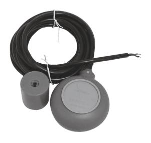
VF Series Float Switch, plastic housing, 5m cable, 1 C/O relay output, IP68 rating
