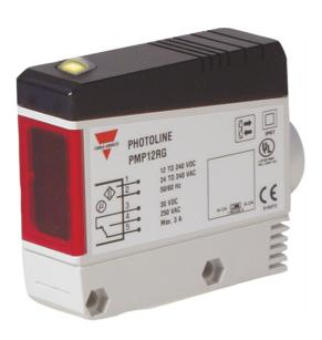
PM Series Photoelectric Switch, modulated infrared light, diffusereflective, plastic housing 25\*65\*81mm, 12 to 240 V DC and 24 to 240 V AC power supply, NC and NO output, adjustable timer, IP67 rating, 1/2" NPT cable gland
