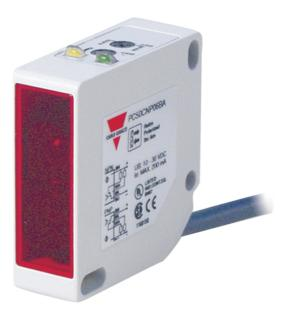
PC Series Retro-reflective Photoelectric Sensor, modulated infrared light, PC/ABS housing, 10 to 30 V DC power supply, transistor NO & NC output, 10m sensing range, output ON, signal stability and supply ON, IP67 rating, M12 plug, with 5m cable
