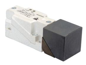
IC Series Inductive Proximity Sensors, thermoplastic polyester housing 40\*40\*118mm, 10 to 30 V DC power supply, PNP NO & NC output, 30mm sensing range, IP67 rating, fully protected, LED-indication for power and output ON
