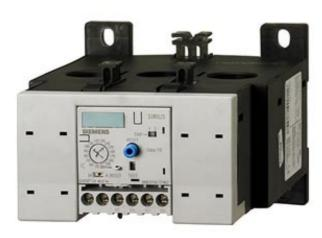
OVERLOAD RELAY 50...200 A FOR MOTOR PROTECTION SIZE S6, CLASS 10 MOUNT. ONTO CONT./ STAND-ALONE MAIN CIRCUIT: THROUGH TRANSF. AUX. CIRCUIT: SCREW CONNECTION MANUAL-AUTOMATIC-RESET
