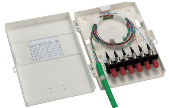
The 601 fiber enclosures are manufactured from UL approved ABS thermoplastic material which is robust but lightweight. The low-profile design provides integral internal fiber management features to ensure the integrity of the cable bend radius and hold splices secure. The product accepts up to 8 fusion splice protectors or mechanical splices. The product is supplied with an identification label for fiber installation traceability. Top or bottom fiber cable entry.
