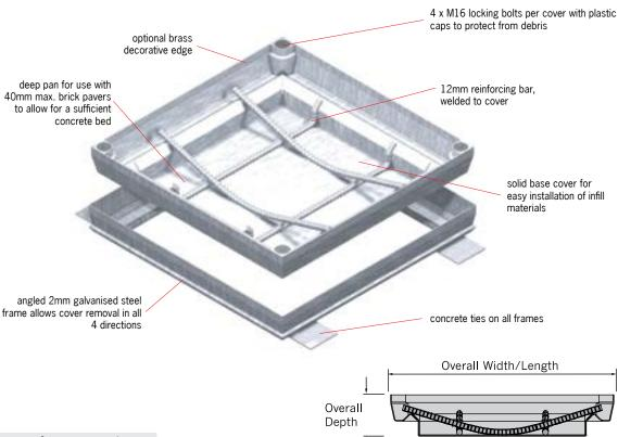
Note: Pavermate® covers are to be filled with concrete to a minimum depth of 45mm. Concrete is integral to the strength of the cover. See page 41 for full details.
